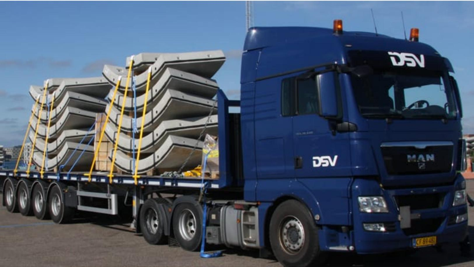
Concrete elements for two tunnel rings loaded on one four axle flatbed trailer
